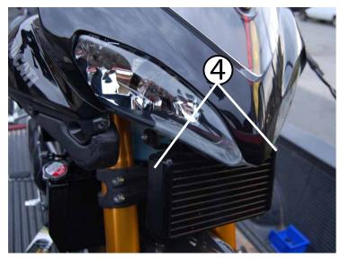
Lightly abrade paint at tape locations with scotchbrite pad. All that is necessary is that the glossy surface be lightly scratched. This will ensure the optimum bond. Using the provided Isopropyl cleaning pad, clean both ends of the cooler, then ensure they are dry before proceeding.
