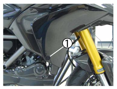
① Using a 4mm allen tool, and a 24mm wrench, remove the indicated fasteners on both sides.
